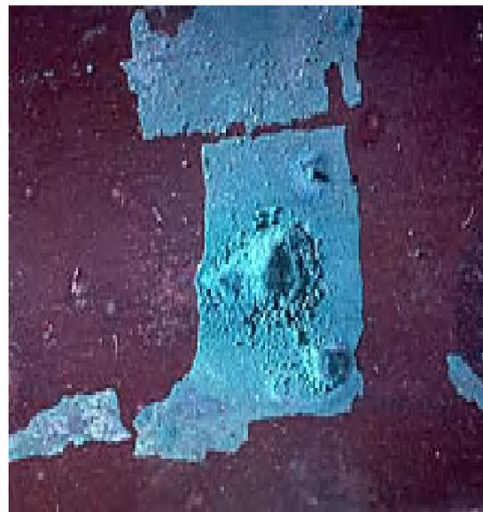
**Fig V.2:** Corrosion externe
