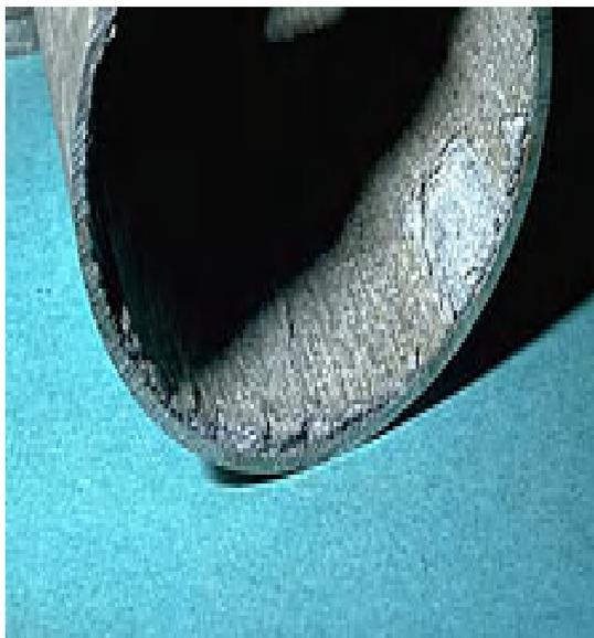
**Fig V.1:** Corrosion interne
