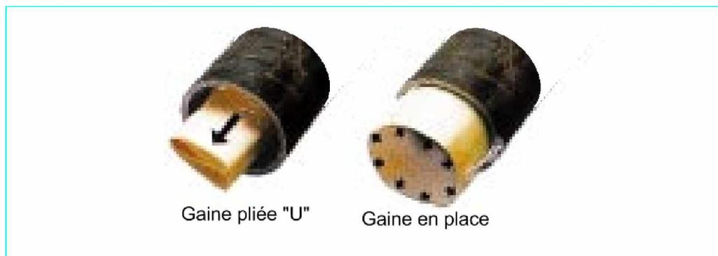
**Figure V.5 – Gainage**
