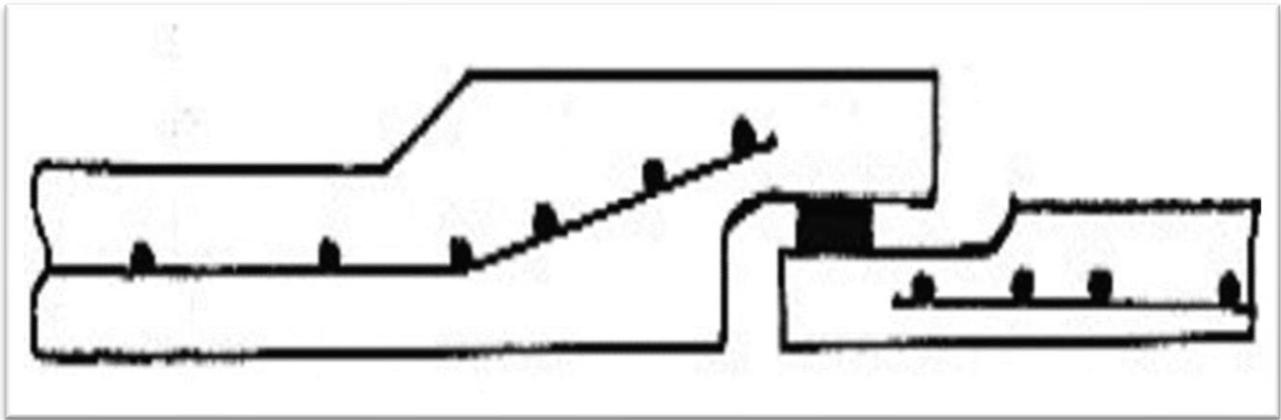
Figure (VI-4) : Joint type Rocla.
