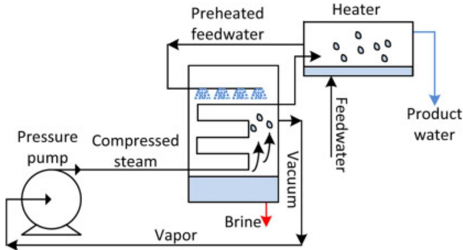
Figure II.2: Illustration of vapor compression distillation (Yousef & Hassan, 2023)
