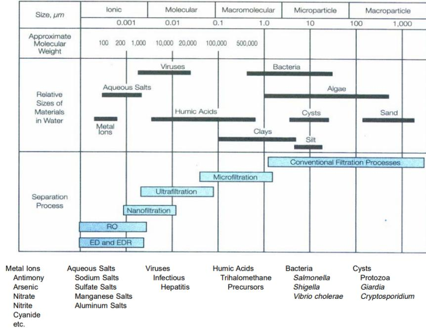
Figure II.5: Filtration capacity of different membrane processes (A.W.W. Association, 1995)
