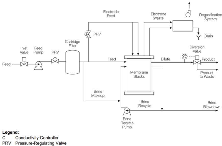
Figure II.10: Electro-dialysis system diagram (A.W.W. Association, 1995)
