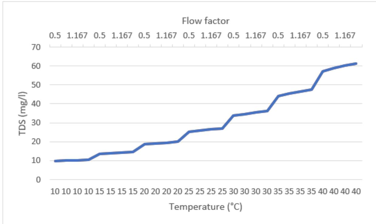
Figure VI.8: Evolution of permeate TDS in function of temperature and flow factor
