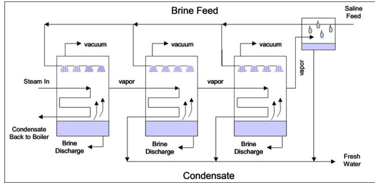
Figure II.1: Diagram of multiple effect distillation evaporator(Saadat et al., 2018)
