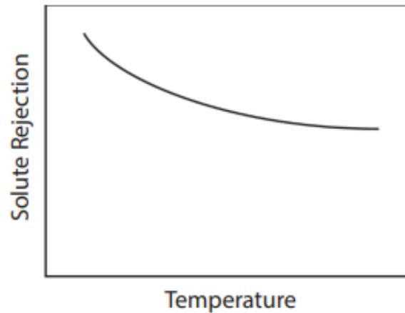
Figure III.13: solute rejection as a function of feed water temperature with constant feed pressure and solute concentration (Kucera, [2023](#))
