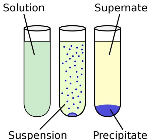
Figure II.3: Illustration of the chemical precipitation process (ZooFari, n.d.)
