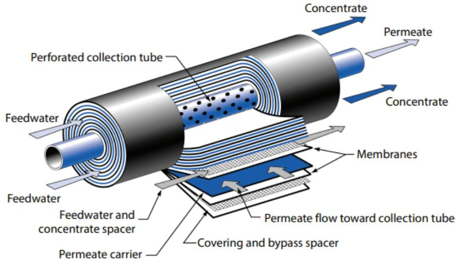
Figure III.9: Spiral wound module example (Kucera, 2023)
