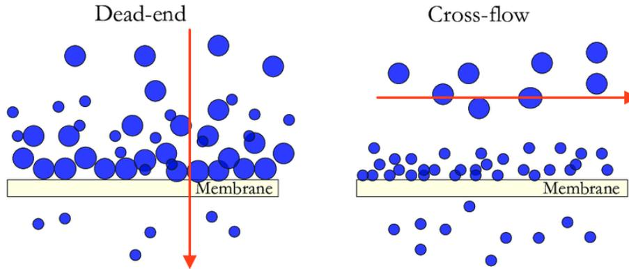
Figure III.2: Dead-end filtration and cross-flow filtration modes (Ruiz-García et al., 2017)
