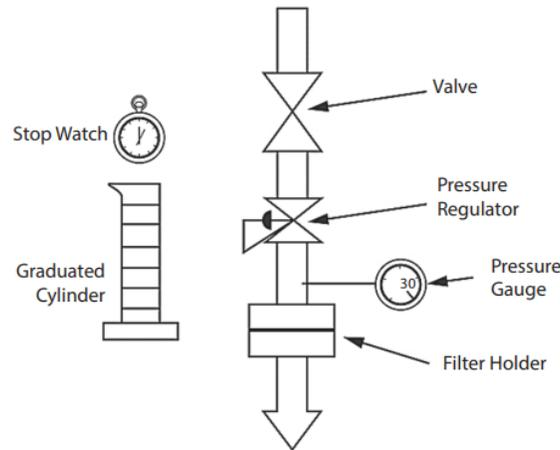
Figure III.4: SDI measuring apparatus at 30 psi (Kucera, 2023)
