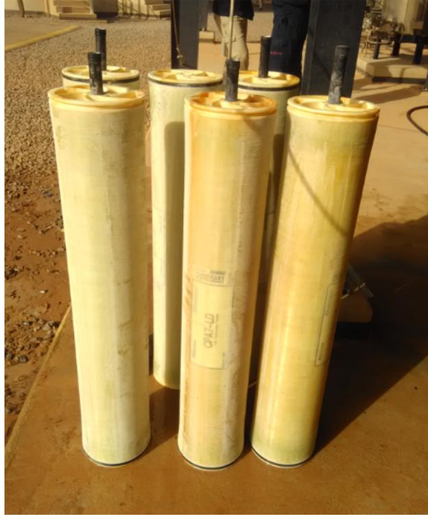
Figure IV.16: Physical damage due to high pressure exposure on the used membranes
