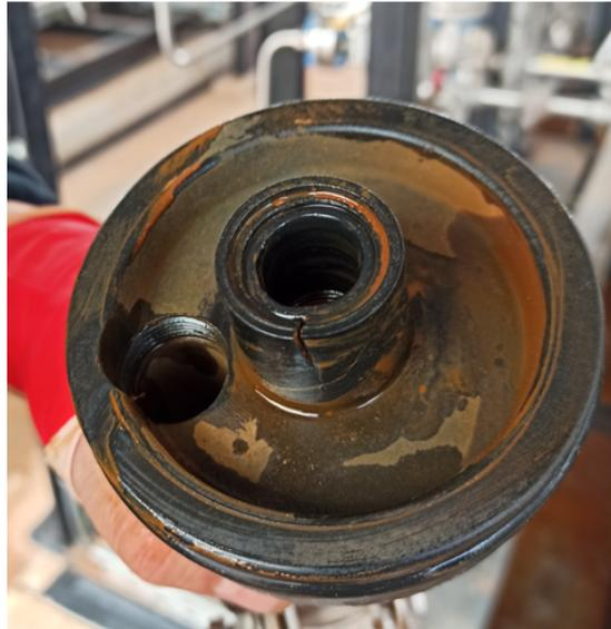
Figure IV.21: Damaged RO2 end cap.
