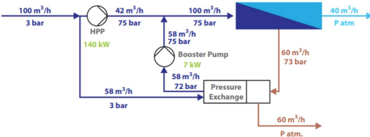
Figure VII.2: Energy recovery pressure exchanger for a single-stage seawater system at 35,000 ppm TDS (Kucera, 2023)
