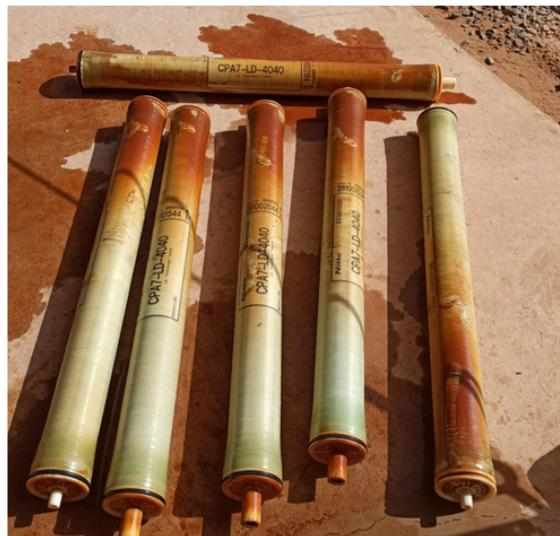
Figure IV.22: Used RO2 membrane with reddish deposits.
