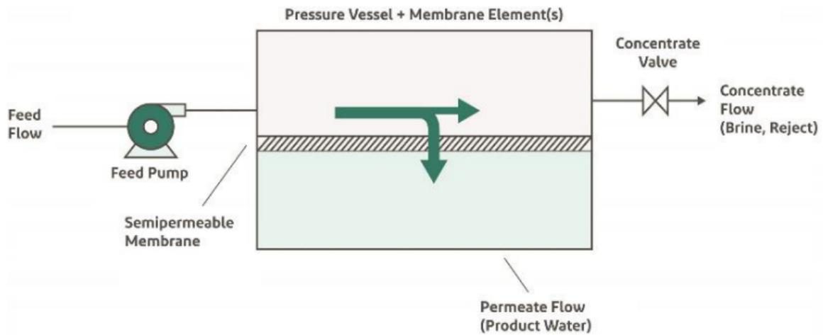
Figure II.8: basic reverse osmosis/nano-filtration process (DuPont, 2023)
