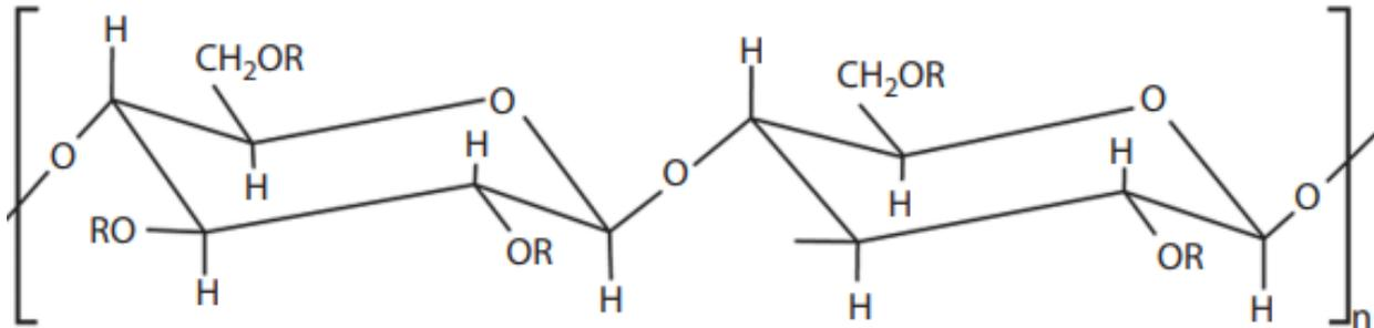
Figure III.6: Chemical structure of a cellulose acetate membrane (Kucera, 2023)
