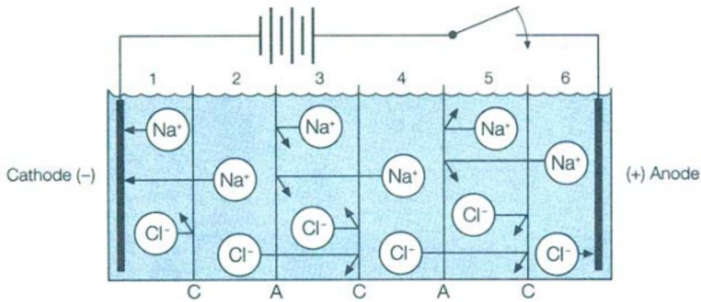
Figure II.9: Electro-dialysis of a basic  $NaCl$  solution (A.W.W. Association, 1995)
