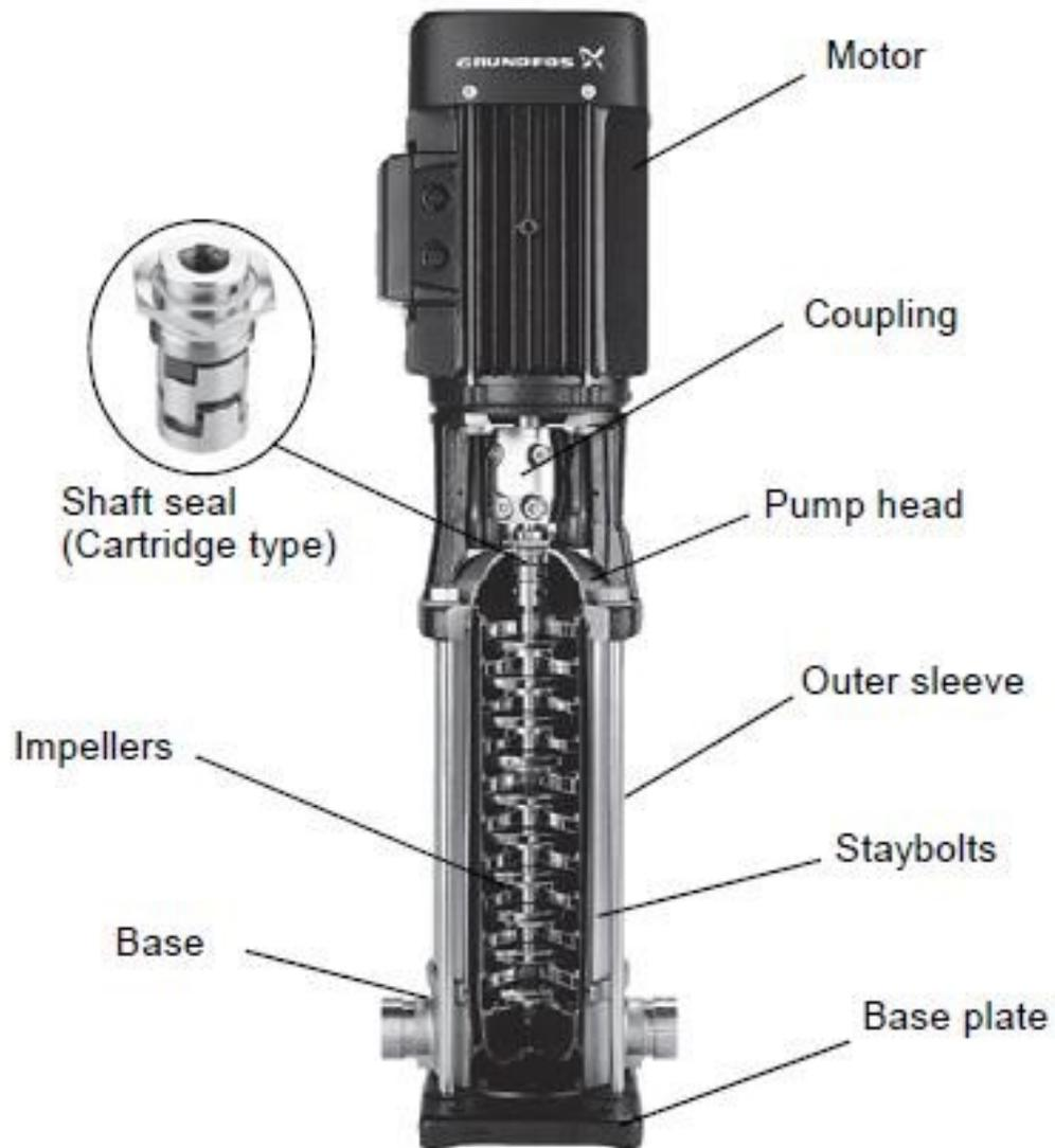
Figure IV.4: RO1 high pressure pumps (Grundfos, 2024)
