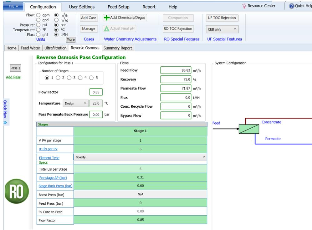
Figure VI.3: WAVE reverse osmosis system design screen
