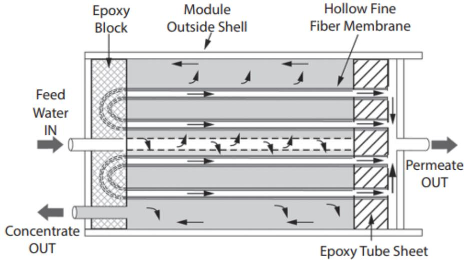
Figure III.8: Simplified example of a hollow fine fiber element (Kucera, 2023)
