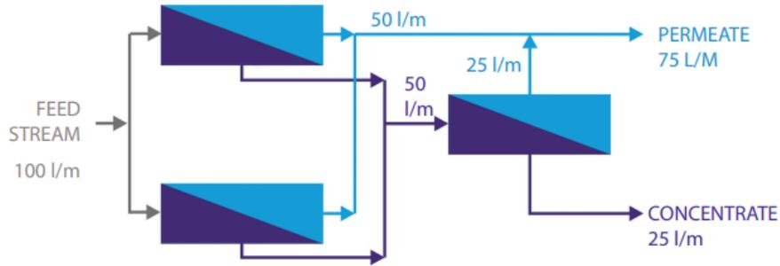
Figure III.11: A two stage, 75% recovery unit (Kucera, 2023)
