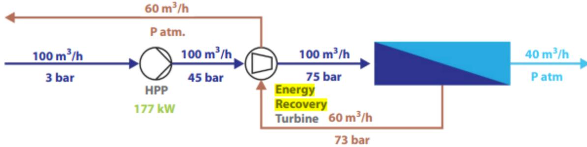
Figure VII.1: 0 Energy recovery turbine for a single-stage seawater system at 35,000 ppm TDS (Kucera, 2023)
