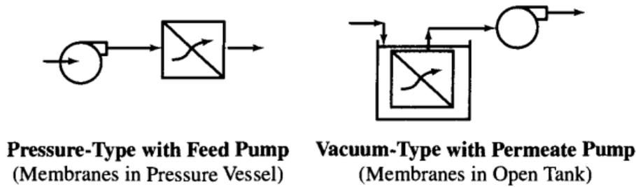
Figure II.6: Pressure-driven processes using feed or filtrate pumps (Baruth et al., 2005)
