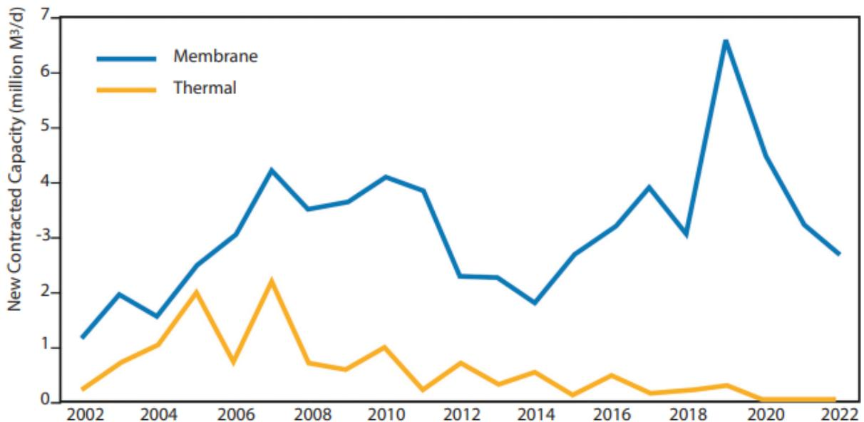
Figure III.1: Thermal desalination vs membrane techniques (Kucera, 2023)
