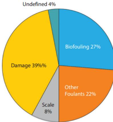
Figure III.14: Failure mechanisms from 99 autopsied seawater membrane elements (Kucera, 2023)
