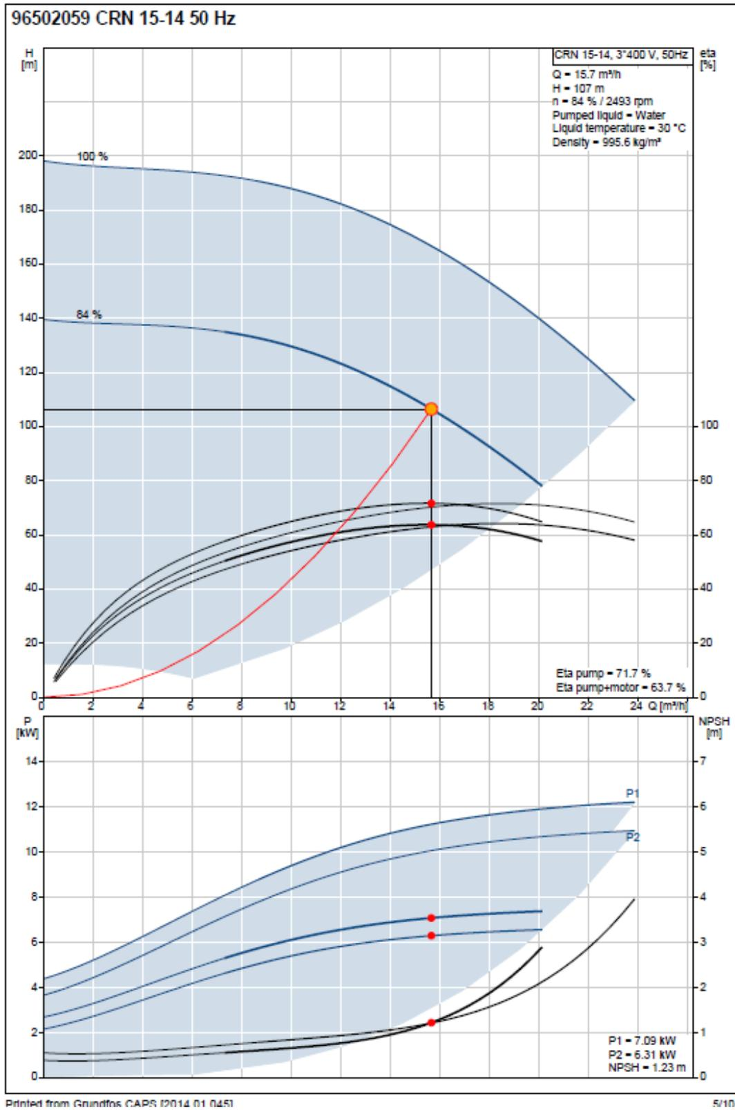
Figure IV.5: RO1 high pressure pumps performance curve (Grundfos, 2024)
