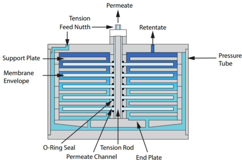
Figure III.7: Example of a plate and frame module (Kucera, 2023)
