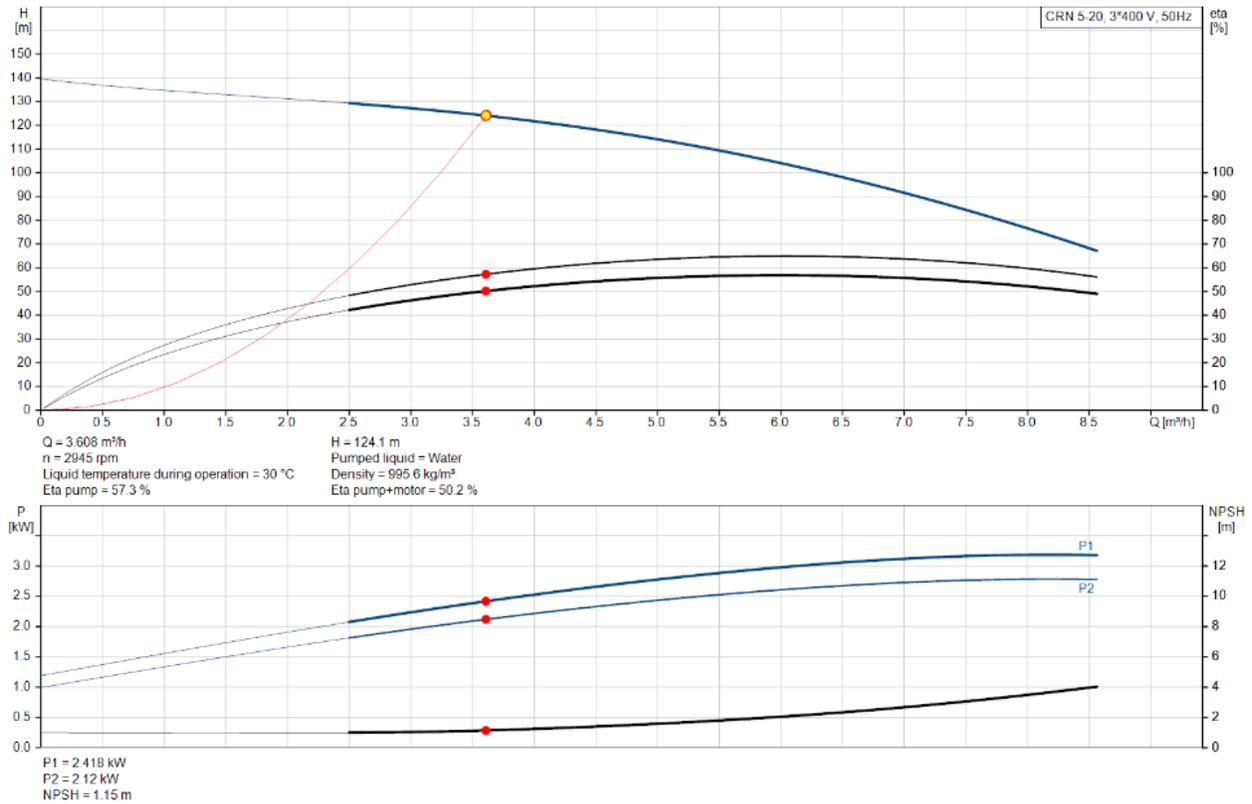
Figure IV.7: RO2 high prssure pump performance curve
