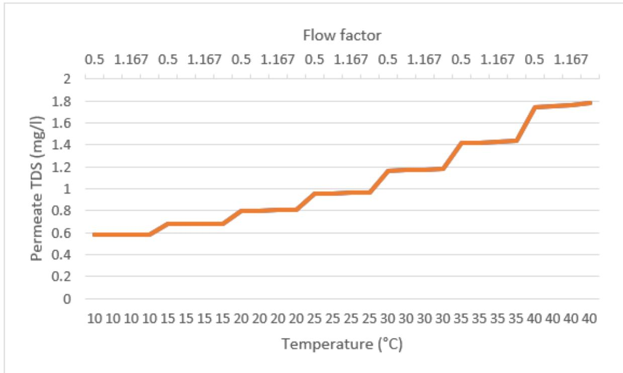
Figure VI.9: Evolution of permeate TDS in function of temperature and flow factor for RO2
