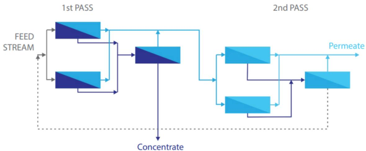
Figure III.12: Two pass RO unit (Kucera, 2023)
