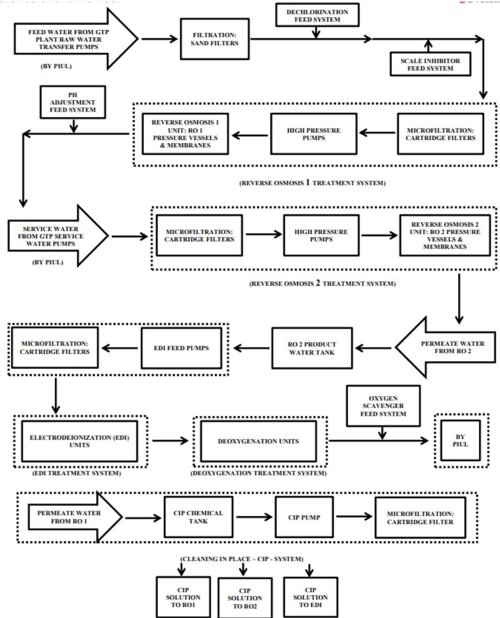
Figure IV.1: Water treatment unit block diagram (EMCO engineering LTD, 2014)
