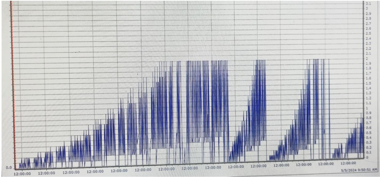
Figure IV.25: Pressure drop for the RO2 cartridge filters.
