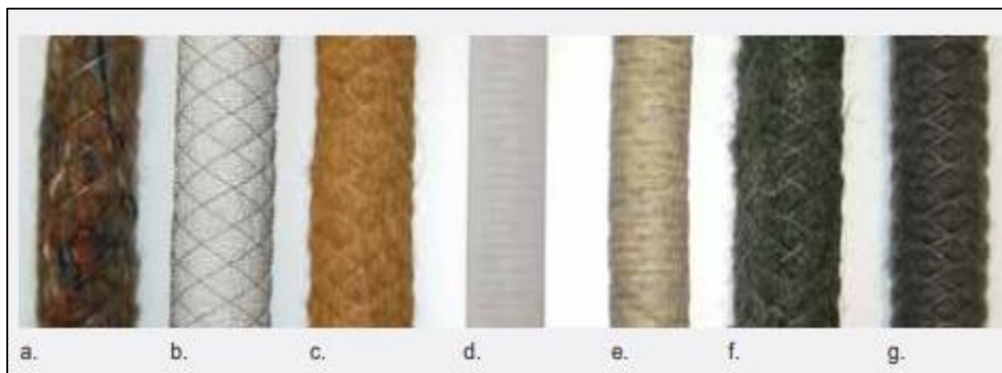
Figure VI.2: Drain envelopes (filters).
