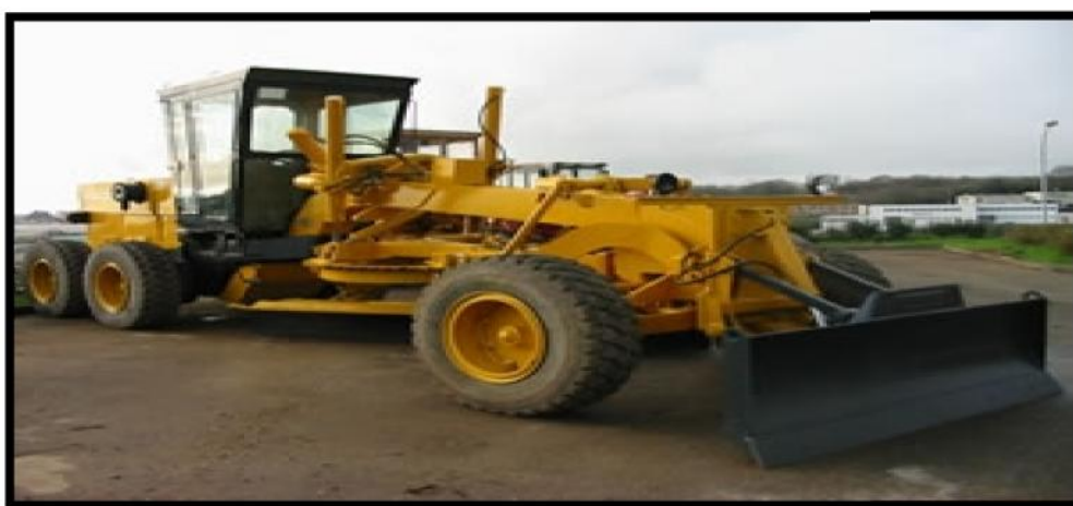
Figure IX.4 : Niveleuse automotrice ;Source ( http://christiandurieux.com/blog/2014/1/13/les-engins-hybrides-ont-la-cote-1 )
